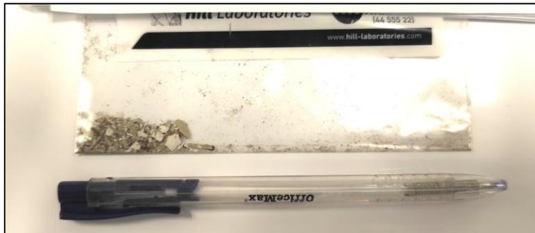
Paint flakes 1mm or less provided with lots of base substrate (non-paint) inclusions.
