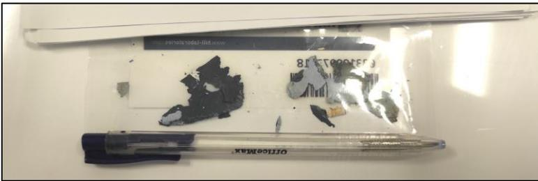
Thick flakes of paint with no inclusion of base substrate (standard pen size for comparison).
