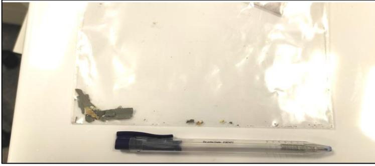
A few very thin paint flakes. 2-3 times more paint would be required to be sufficient.
